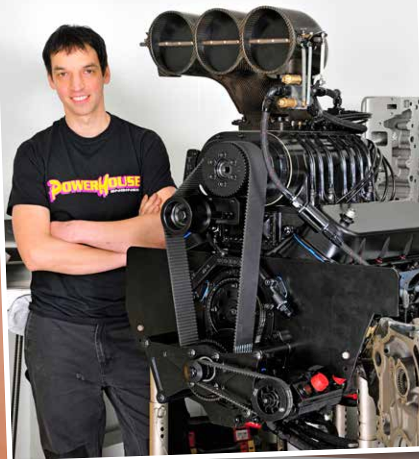
John with the dry-sumped 477ci monster he's building for Mick Brasher's new car
